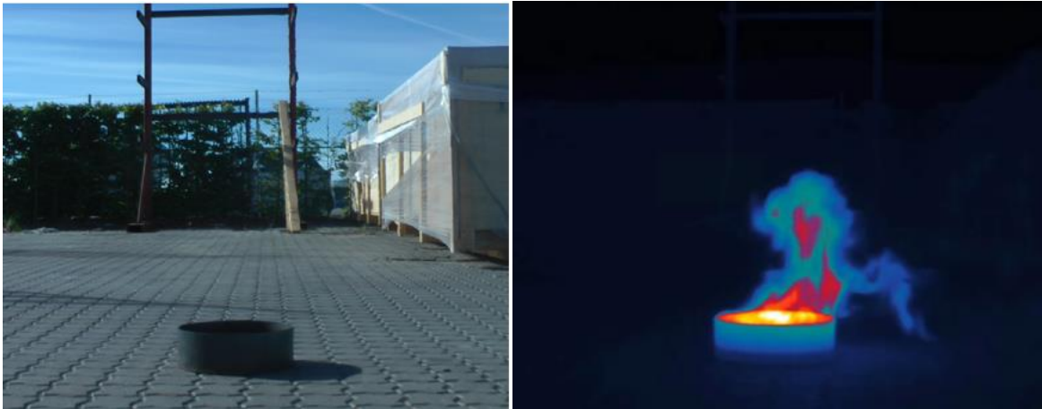
Figure 1. Left: Methanol burning invisibly on a sunny day. Right: Thermal camera imaging
