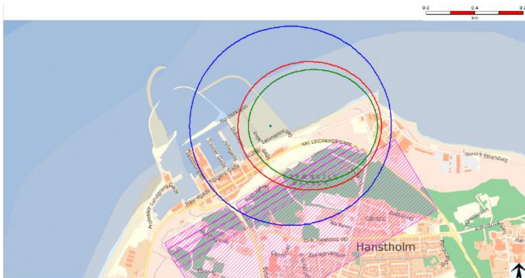
Figure 18. SC-1. Cloud maximum footprint contour of 84000ppm on the map of Hanstholm port with prevailing west winds at the ground level.
